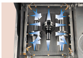
Automatic washing from 18 nozzles.
